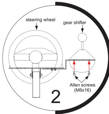
Put your wheel on the main plate and drive two Allen screws (M6x16) to fix it firmly. Drive another two screws (M6x16) to fix the gear shifter to the gear shifter plate.
